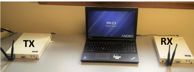
Fig. 3: Software defined radio testbed
